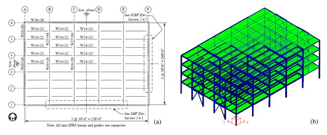
Figure 4-1. Steel building example: (a) building plan [30], (b) 3D elastic model developed in S-FRAME.
