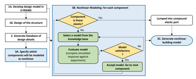
Figure 3-1. Nonlinear modeling process within the proposed framework.
