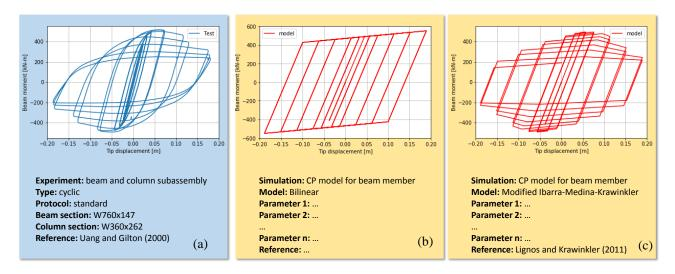
Figure 3-2. Example of an instance of model validation: (a) actual behavior, (b) and (c) simulations.
