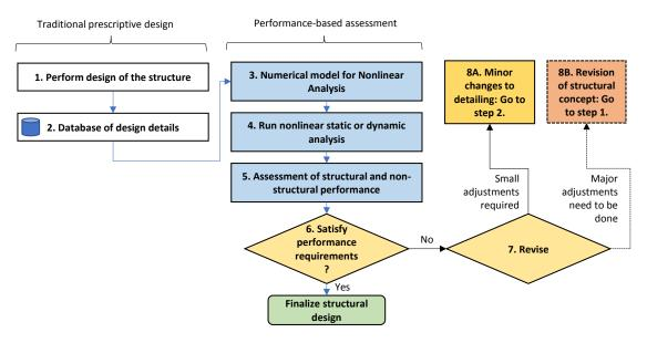
Figure 1-1. Overall design process in Performance-Based Seismic Design of buildings.
