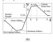
Figure 2-1. Backbone curve: (a) monotonic and cyclic backbones [10], (b) schematic definition [14].
