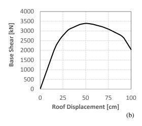
Figure 4-2. Framework application: (a) Selected structural components, (b) nonlinear static analysis result.
